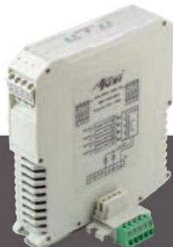
**i** To supply sensors with channel-to-channel isolation with power, an appropriate number of isolated sources is required. WAD-POW-BUS Module forms 8 channels with channel-to-channel isolation in one box. For instance, we obtain 8 input channels being open on a channel-to-channel basis with two WAD-POW-BUS modules.
